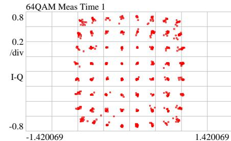
*Constellation display shows symbol points only, revealing problems such as compression (shown here).*
