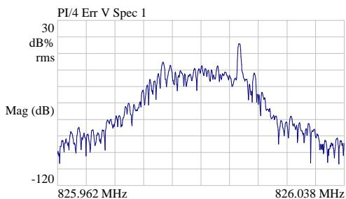
*Power supply ripple appears as EVM spur, offset from carrier by 10 kHz.*
