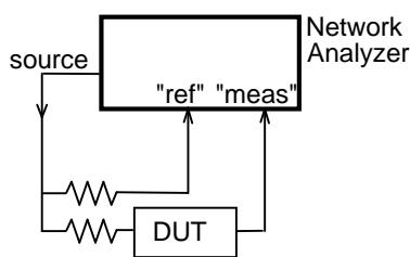
*In traditional two-sided network analysis, the DUT's input signal is carefully measured so that any imperfections in the source signal can be mathematically removed.*
