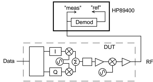
With an 89400, the DUT input signal doesn't need to be supplied or measured, because it is calculated (regenerated) from the measured signal, and is thus already in ideal form.
