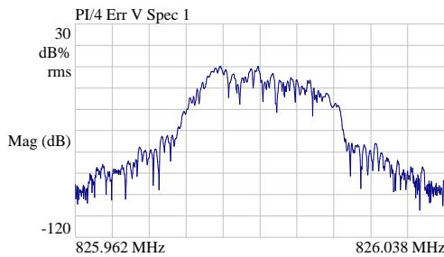
*Interference from adjacent (lower) channel causes uneven EVM spectral distribution.*
