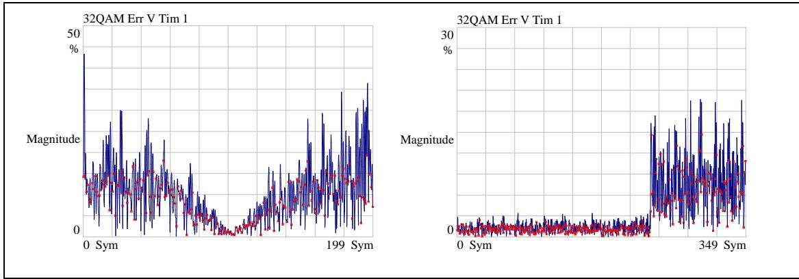
*V-shaped EVM plot due to incorrect symbol clock rate.*
