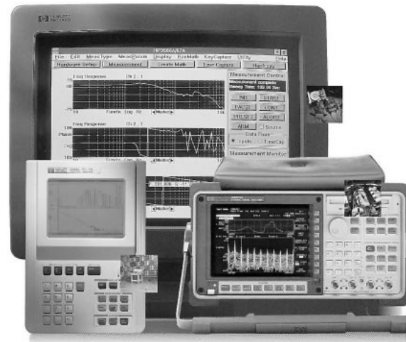
Figure 6.1-1 Hewlett-Packard DSAs representa- tive of the hand- held, benchtop and systems types.
