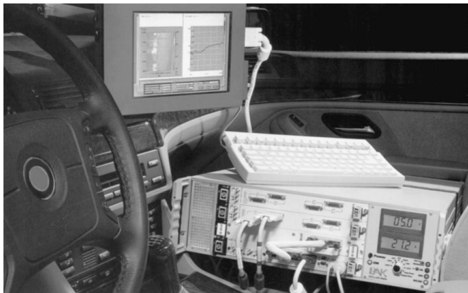
Figure 2: The new PAK-Mobil system provides psychoacoustic capabilities in a portable package.
