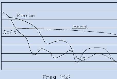
Figure 2: The shape of the impact pulse and its frequency profile depend on the hammer tip you've chosen.
