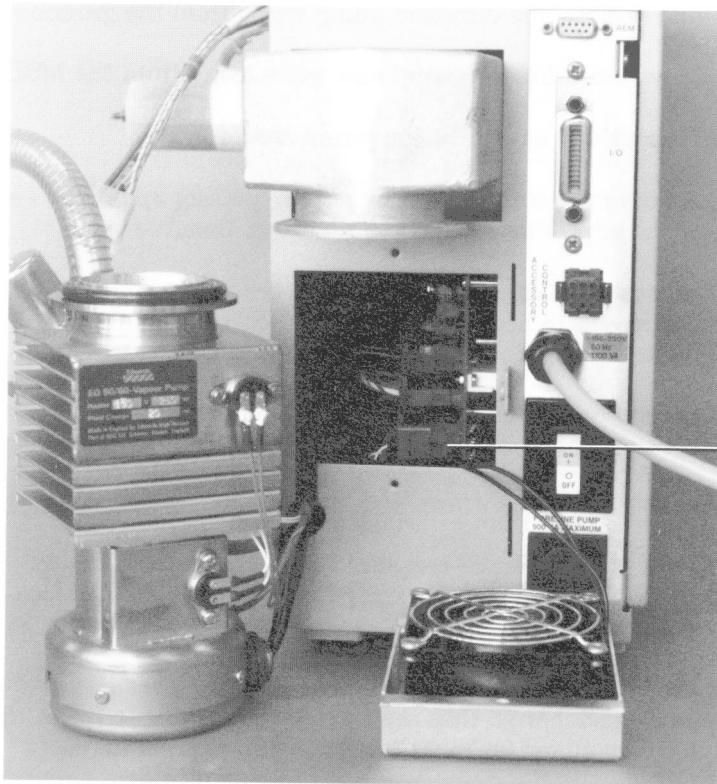
Figure B-37. Diffusion pump wiring connector
