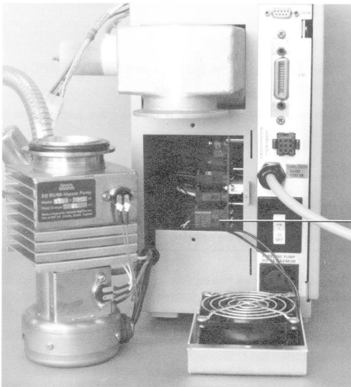
Figure 6-6. Disconnecting the diffusion pump wiring
