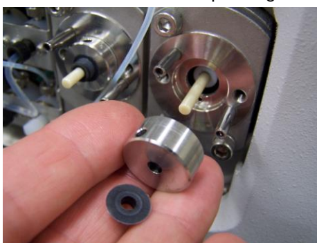
Figure 7. Piston guide and pump seal.
