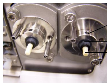
Figure 4. Pump heads removed with pump seals remaining on the piston.
