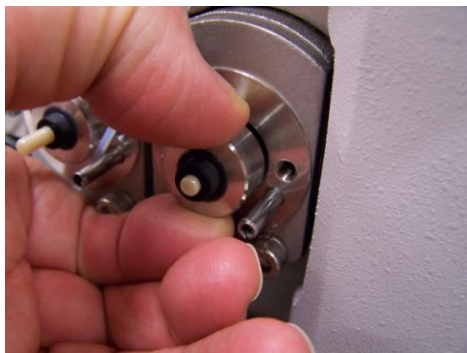
Figure 5. Pulling the piston guide to remove the seal.
