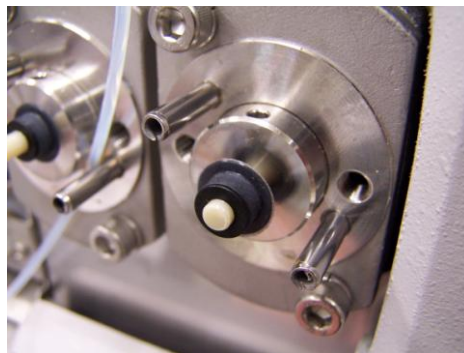
Figure 6. Pump seal after being pushed by the piston guide.
