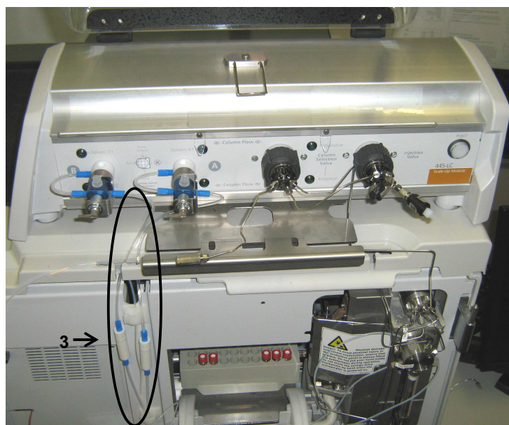
Figure 5: Connecting the debubbler line to the pumps
