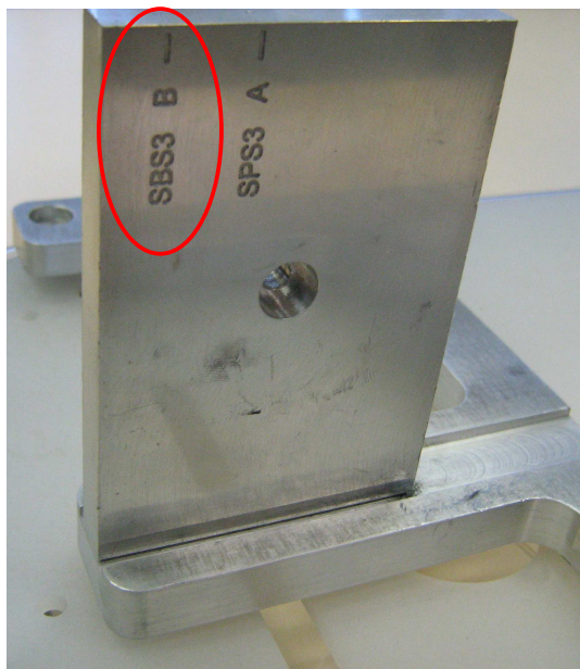
Figure 16: Calibration Point B in the Alignment Tool
