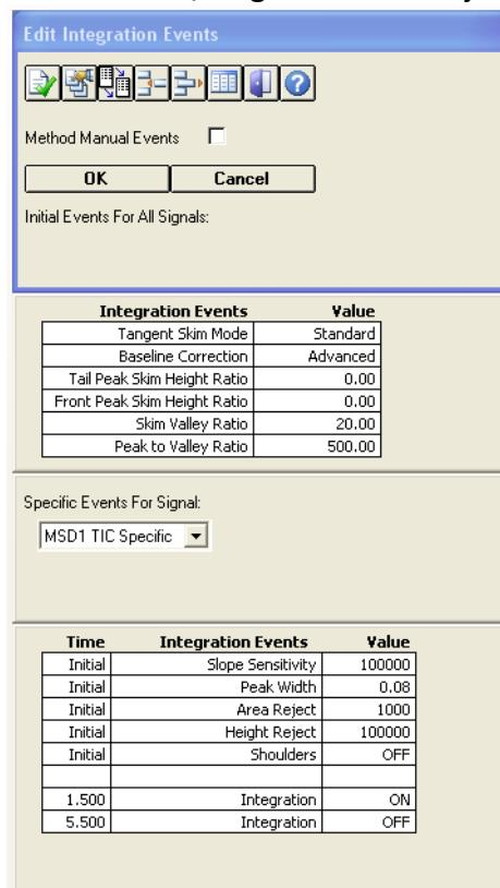
n. Save the method as “Analyt\_Basis\_Short” and create a sequence of 3 injections.
