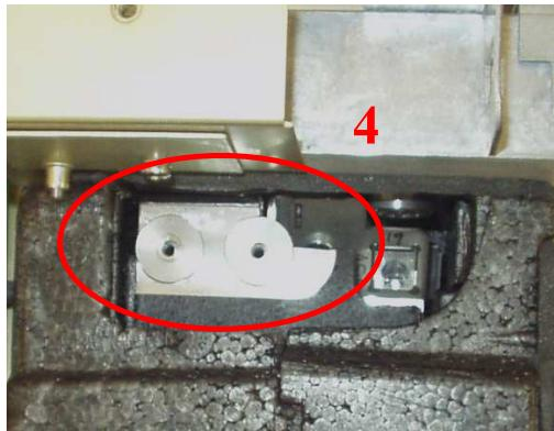
6. Carefully place the Vis option over the opening making sure that the lens fits nicely into the hole leading to the optics. Once the Vis option is in position (5), lightly tighten the provided screws.
