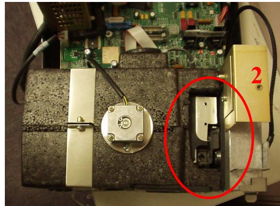
3. Once the foam or the metal plate has been removed you will see a hole looking down into the optics (2) on the front side of the optics (the side closest to the front panel), and 2 screw holes that you will use to mount the Vis option on the back side of the opening (side furthest from front panel)
