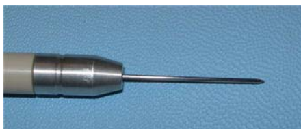
Figure 36 APCI corona needle after cleaning.
