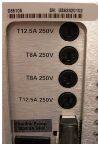
Figure 76 AC Board fuses
