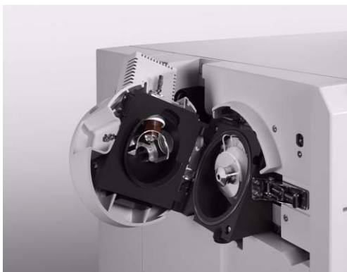
Figure 17 Opened electrospray Agilent Jet Stream Technology spray chamber
