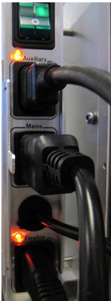
Figure 7 Pump expander box ports.
