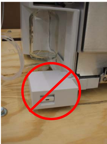
Figure 6 Do not lift from under power switch bracket
