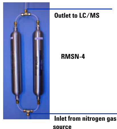
Figure 11 Gas filter connected in parallel
