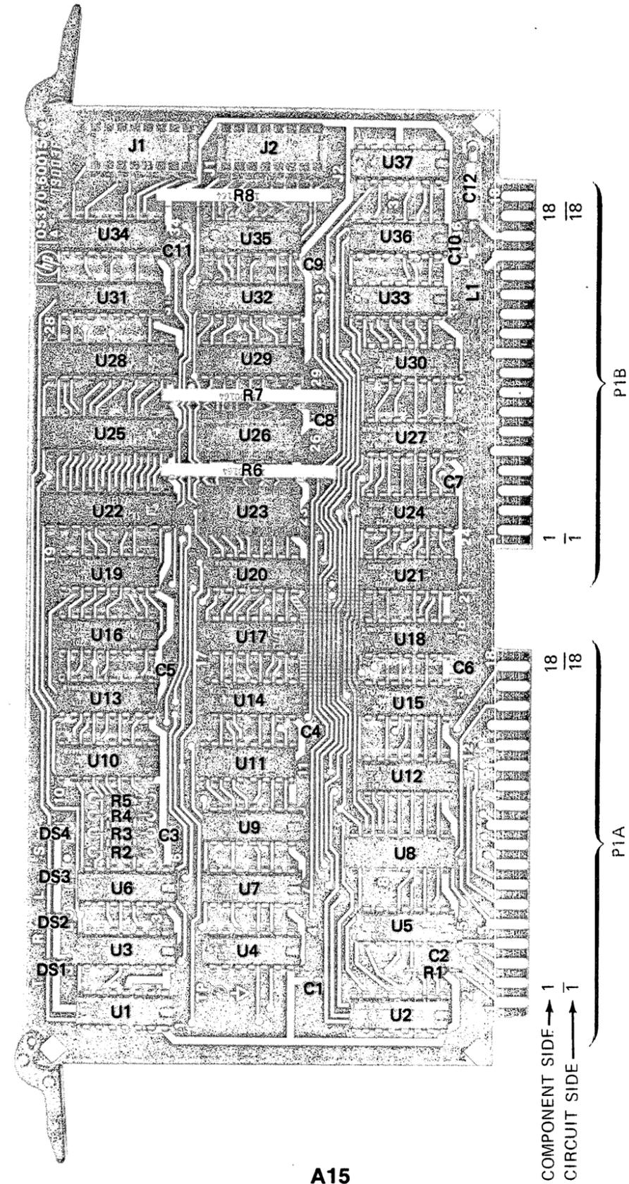
Part of Figure 8-25. A15 HP-IB Interface Logic Assembly
