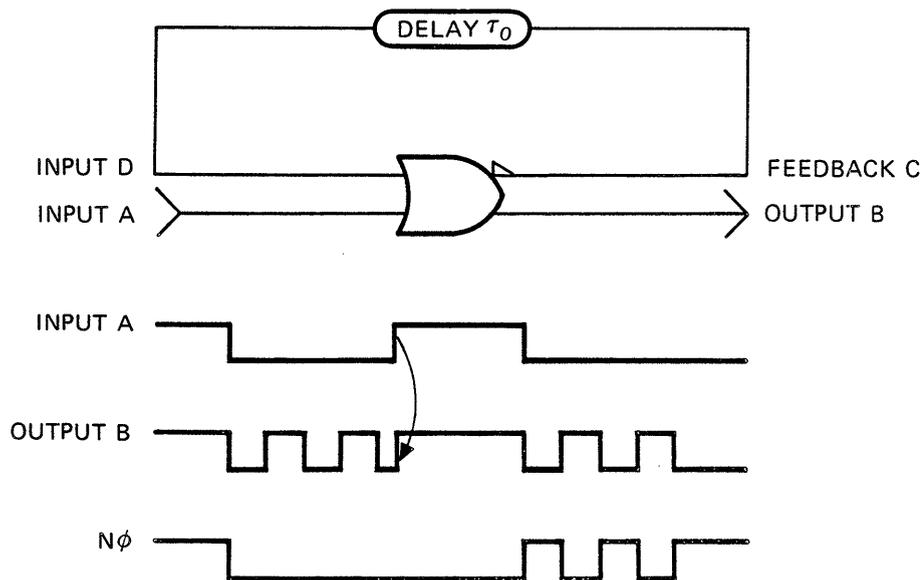
*A Simple Startable Oscillator With Input and Output Signals*
