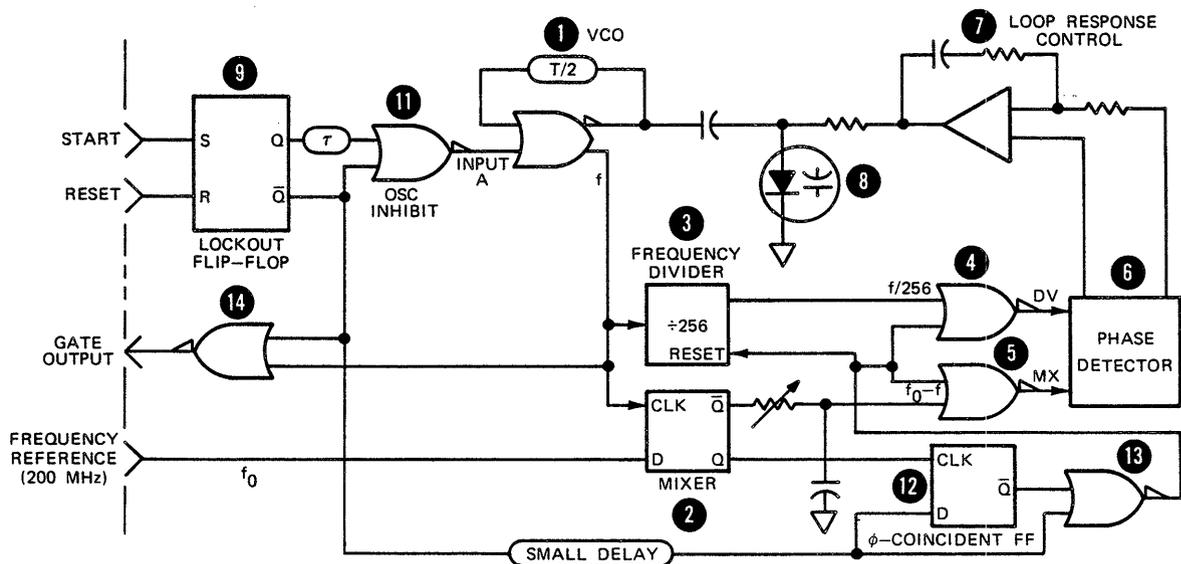
8-227. The new phase of the oscillator is immediately translated to a new phase of the beat frequency through the mixer. But this new phase is momentarily withheld from the phase detector through the signal S, which goes high as gate 13 senses the arrival of the input through  $\bar{Q}$  of lockout flip-flop 9. The signal S causes both DV and MX to go low, disabling the phase detector. The same signal also resets the divider 3 and holds it at 00.
