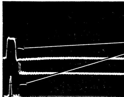
ADJUST PULSE GENERATOR TO ALIGN THESE EDGES
