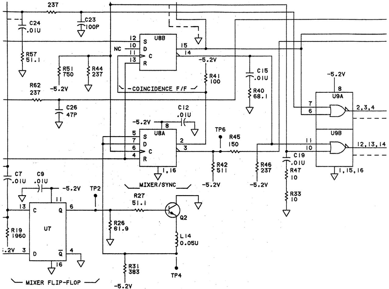
The schematic above is the center portion of the A19/A20 assembly for series 1748A. Substitute this for the same portion of the schematic in *Figure 8-24*. This action will change the A19/A20 schematic (05370-60119 Series 1812A) to match the 05370-60019 (Series 1748A) assembly.
