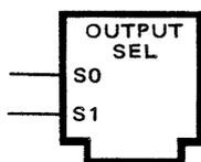
Output selector control block. This symbol is used with a block symbol having multiple outputs to form a decoder. The selection lines enable the output designated 0, 1, ..., n of each block by means of a binary code where S0 is the least significant digit. If the 1 level of these lines is low, polarity indicators ( ▽ ) will be used.
