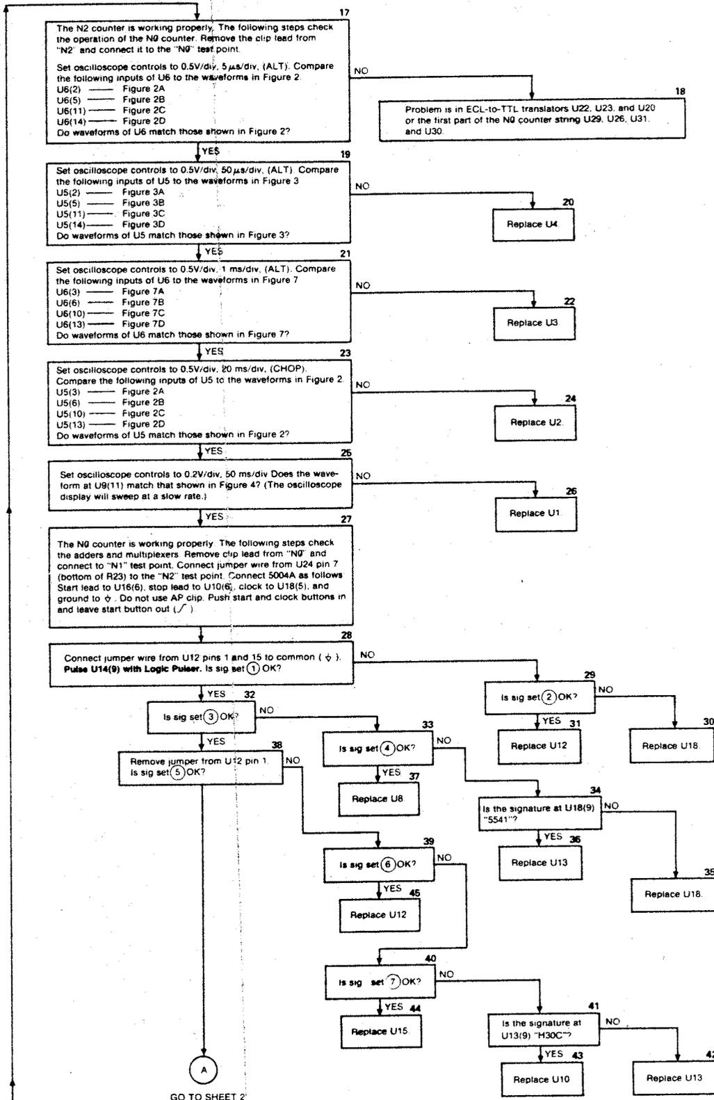
Figure 8-12. A17 Assembly Troubleshooting Flowchart (Sheet 1 of 2)
