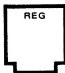
Register control block. This symbol is used with an associated array of flip-flop symbols to provide a point of placement for common function lines, such as a common clear.
