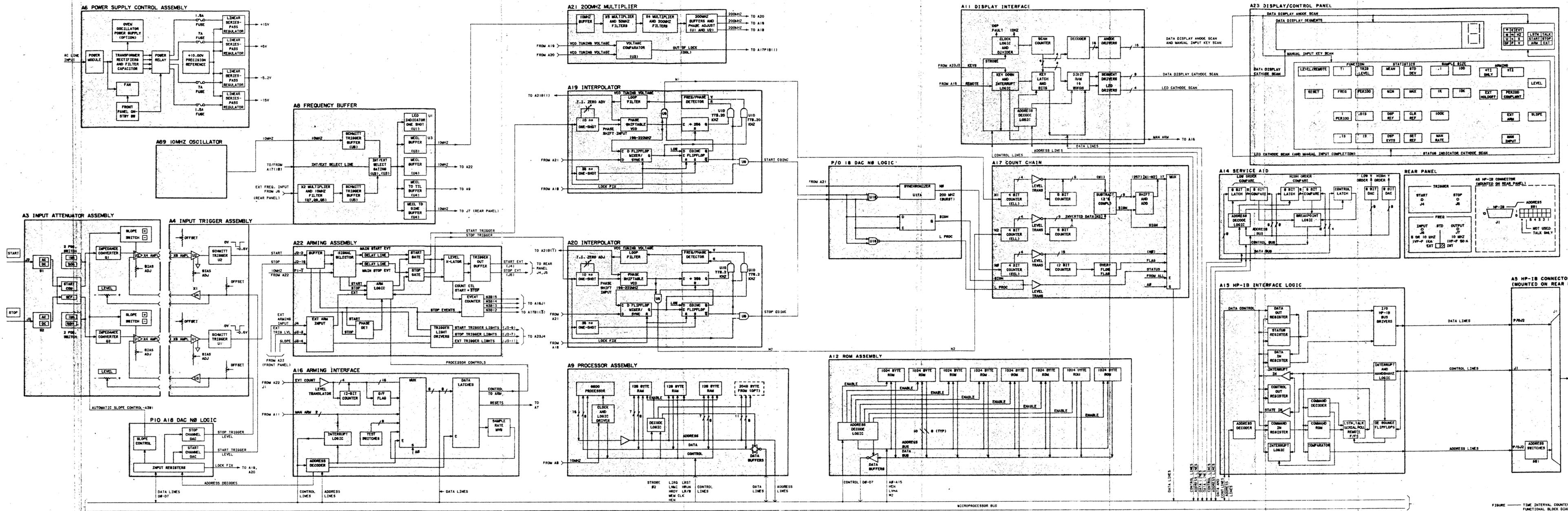
FIGURE 8-16. TIME INTERVAL COUNTER FUNCTIONAL BLOCK DIAGRAM (8570A)
