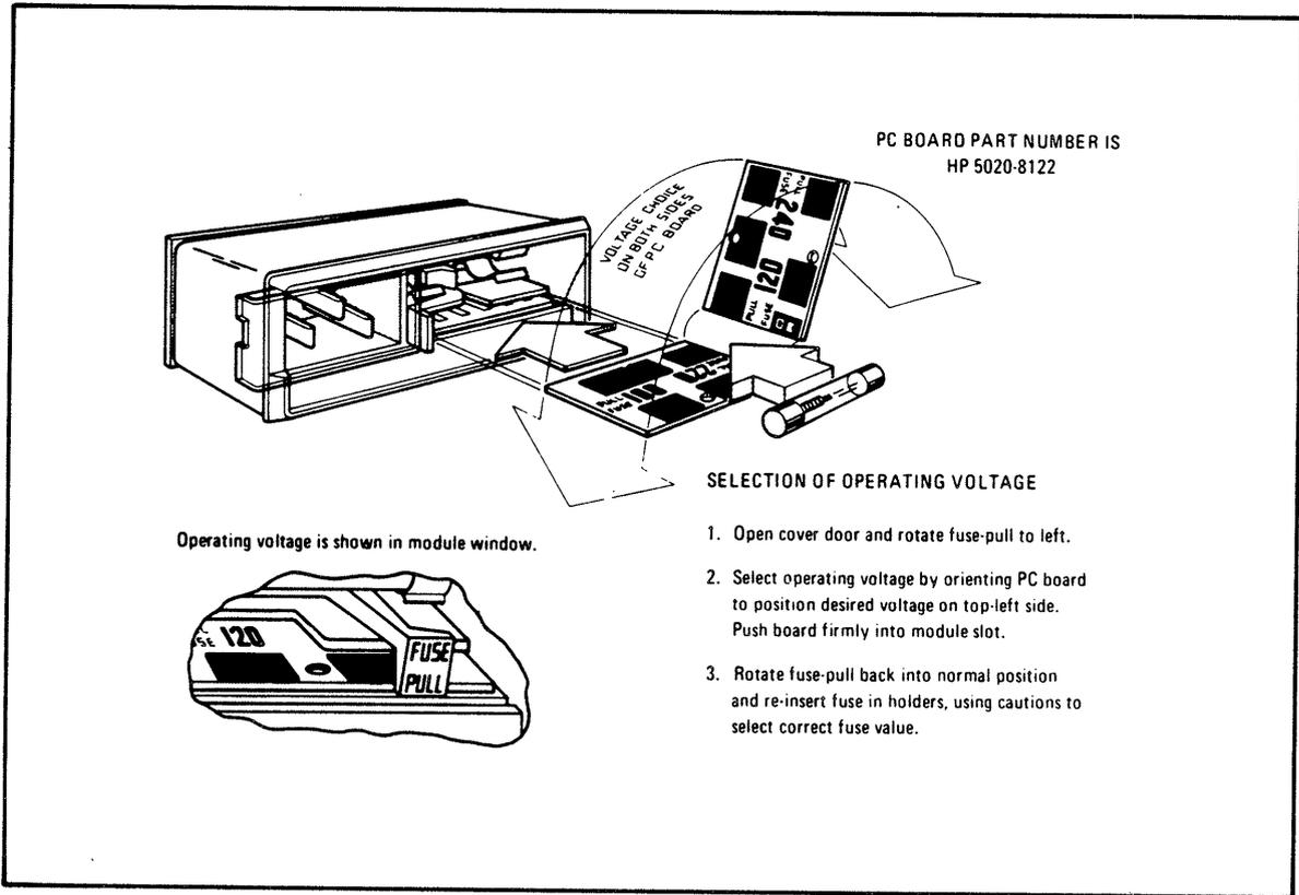
Figure 2-1. Line Voltage Selection
