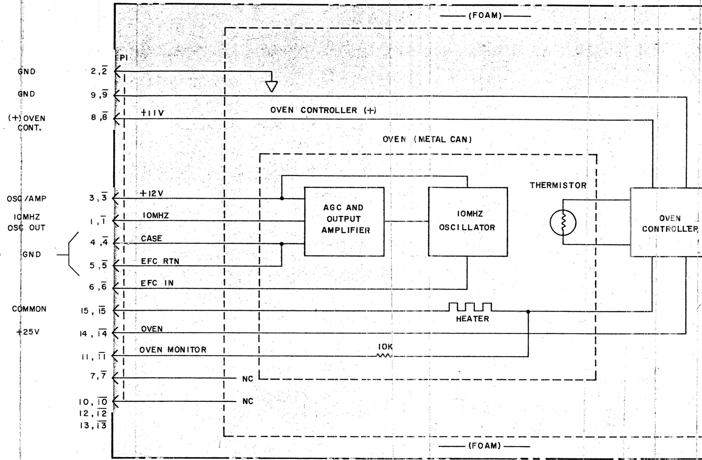
Figure 8-34. A69 10 MHz Oscillator (Mode 1)
