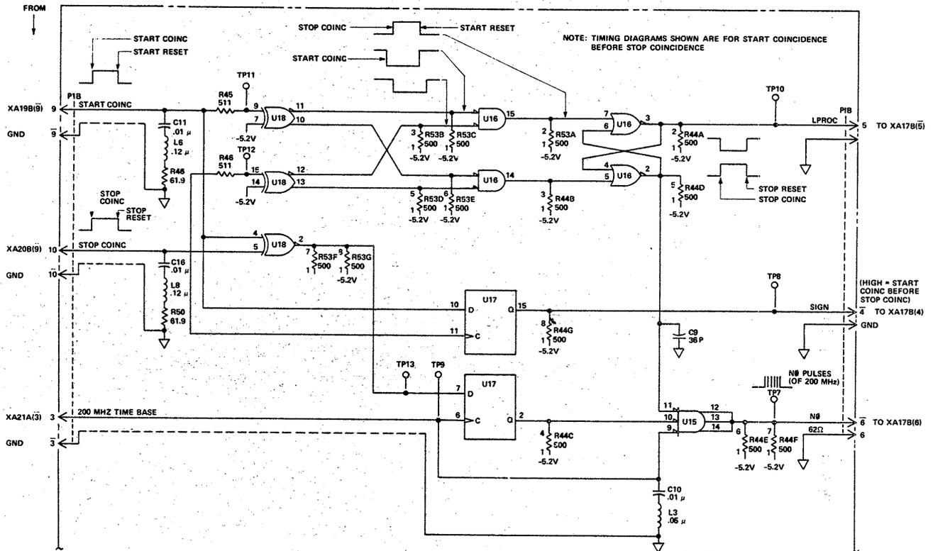
The schematic above is N0 portion (right side of the schematic) of the A18 assembly. Substitute this for the right side of the schematic in Figure 8-23. Notice the inputs and outputs of the assembly board are the same.
