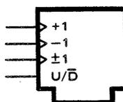
Counter control block. The symbol is used with an array of flip-flops or other circuits serving as a binary or decade counter. An active transition at the +1 or -1 input causes the counter to increment one count upward or downward, respectively. An active transition at the +1 input causes the counter to increment one count upward or downward depending on the input at an up/down control.
