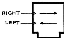
Shift register control block. These symbols are used with any array of flip-flop symbols to form a shift register. An active transition at the inputs causes left or right shifting as indicated.
