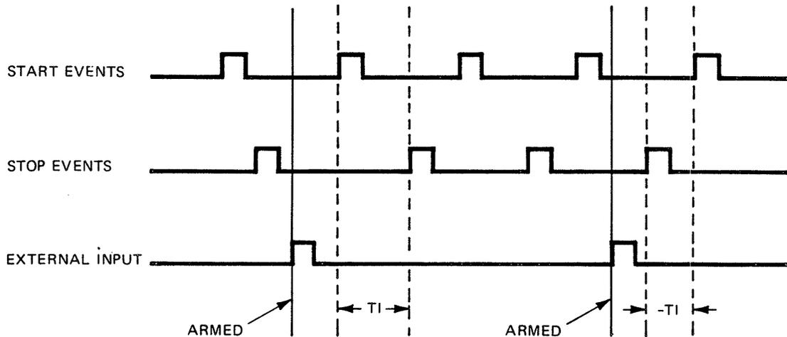
3-20. **EXTERNAL ARM/EXTERNAL HOLDOFF.** To operate the counter in the EXTERNAL HOLD-OFF mode, press the EXT HOLDOFF switch on the front panel. The selected trigger edge at the external input then arms the counter. The next START input pulse begins the measurement. The STOP pulses are held off as long as the external input holdoff is present as illustrated in the diagram.
