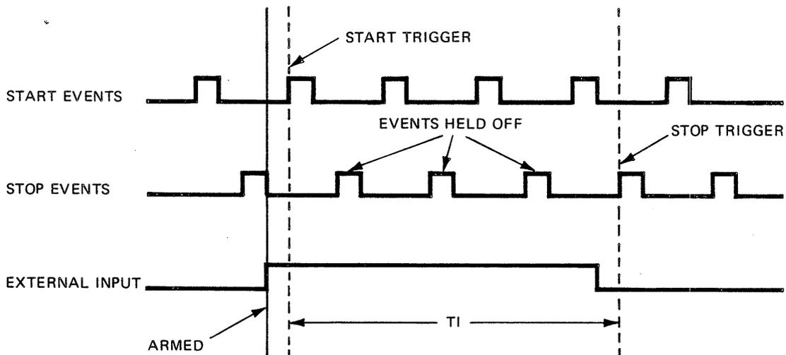
The number of events held off are counted and stored by the 5370A and can be displayed by pressing the DSP EVTS switch on the front panel.
