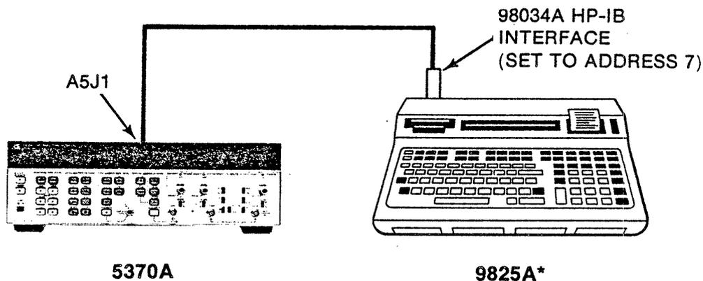
\*9825A should have either the 98213A General I/O-Extended I/O ROM or the 98214A Plotter-General I/O-Extended I/O ROM.
