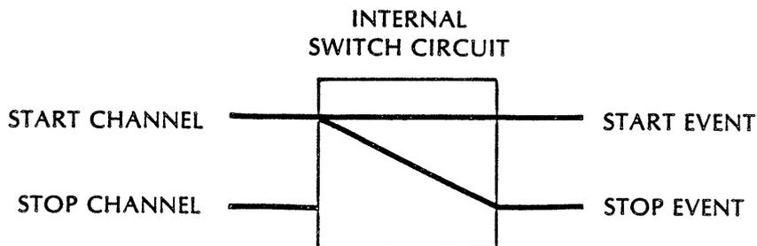
IN4 Input selection for operator convenience in switching input to different channels. START event = STOP channel input, STOP event = START channel input.
