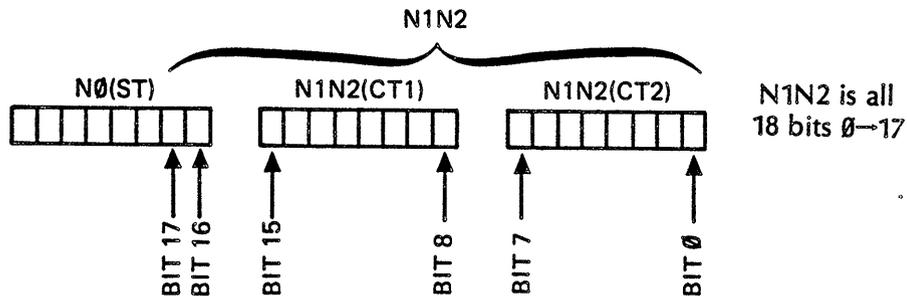
N1N2 actually represents the internal calculation of  $257(N1-N2)$ . This is done in preparation of solving the equation:  $T.I. = 5 \left[ \frac{257}{256} (N1-N2) + N0 \right]$  ns. The number 257 in  $257(N1-N2)$  is part of the ratio  $257/256$ .
