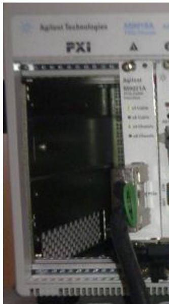
(M9021A Mounted on Slot-1 of M9018A chassis)
