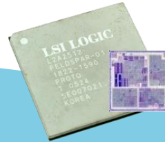
ASIC enabled real-time amplitude and phase corrections
