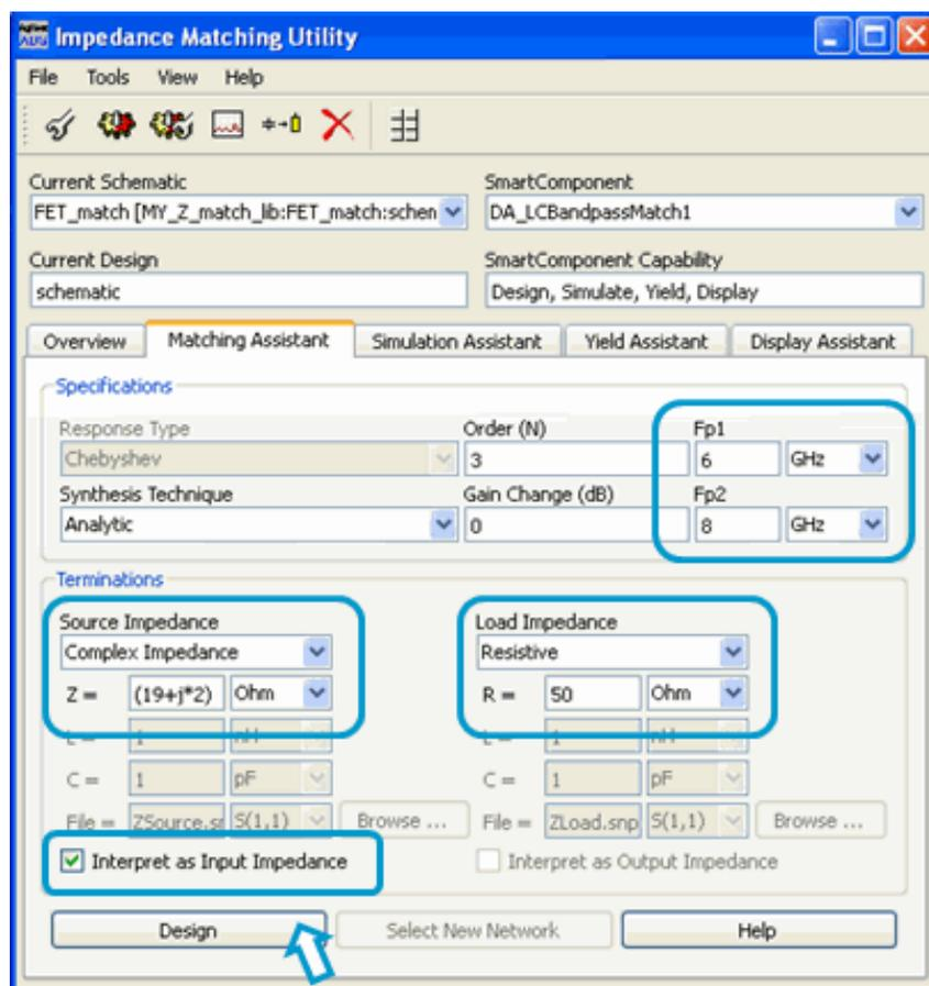
**NOTE:**  $19+j*2$  is an approximate value of load impedance from the load pull results (lab 1). This value will be seen by the amplifier output, and 50 ohms will be seen by the next stage. In other words, this is transforming the optimum load match to 50 ohms..
