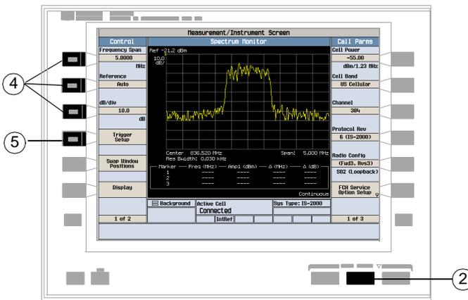
The spectrum monitor is displayed with the default settings as shown above. The center frequency is initially set at the expected frequency maintained by the test set's base station emulator. The Swap Window Positions (**F5**) key is only displayed when other measurements are active at the same time as the spectrum monitor.
