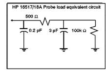
Input Capacitance 0.2 pF and then, through 500 ohms, 3 pF
