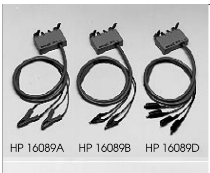
HP 16089A/B/C/D Clip Leads Connector type: A/B/C: Kelvin, D: Alligator Frequency: 5 Hz to 100 kHz Cable length: A/B/C: 0.94 m, D: 1.3m
