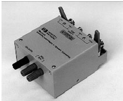
HP 16314A Balanced/Unbalanced 4-Terminal Converter Frequency: 100 Hz to 10 MHz Connectors: 4 BNCs (unbal.), 2 signal terminals & 1 ground terminal (bal.) Characteristic Z: 50 ohms
