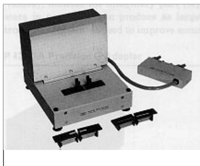
HP 16047B Axial and Radial Test Fixture with Safety Cover Frequency: \leq 2 MHz Maximum dc bias supplied from instrument: \pm 35 V
