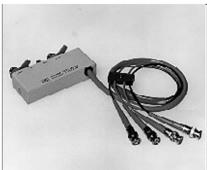
HP 16048A/D/E BNC Test Leads Frequency: A: \leq 30 MHz, D: \leq 30 MHz, E: \leq 1 MHz Cable length: A: 0.94m, D: 1.89m, E: 3.8m Maximum dc bias: \pm 300 V
