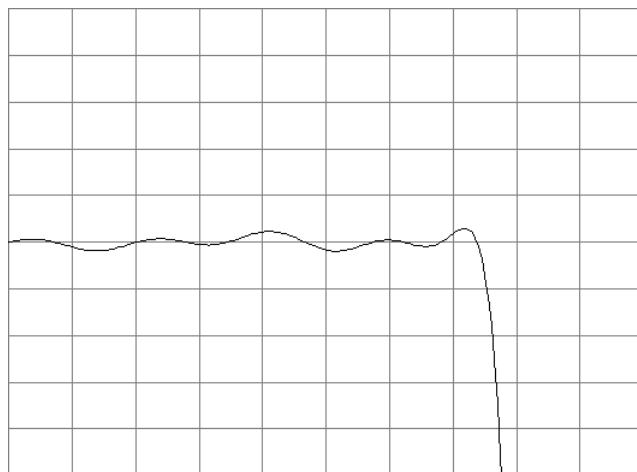
Figure-11. Deviation from linear phase for compensated digital alias filter of bandwidth <<4 MHz. Vertical scale is 0.1°/div. Horizontal scale is .05 of digital filter output sample rate.
