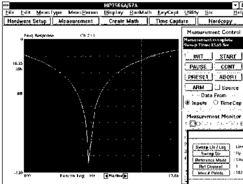
Measuring systems like this notch filter require the high dynamic range of swept sine.
