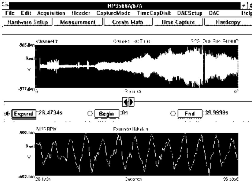
You can look at the entire time capture file channel by channel. The top display is the envelope of the complete time capture. To zoom in for a closer look use the Expand Marker. The bottom trace shows the area selected with the Expand Marker. To identify corrupt data, overloaded portions of the time capture are shown in red.
