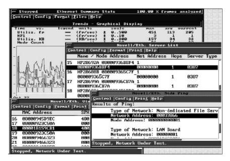
With statistical network performance measurements continuing to run in the background, the Internet Advisor for LAN uses stimulus/response tests to list all active Novell servers and clients, and to verify connectivity.
