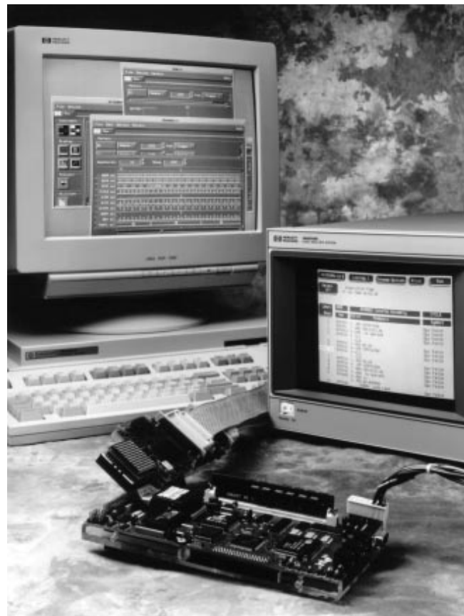
Figure 6. Easily connect to your target system with an HP preprocessor for your specific microprocessor or bus.
