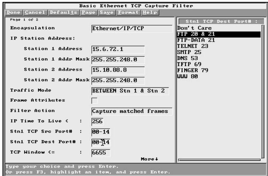
High performance capture filters allow you to focus on data traffic that is related to the problem at hand.
