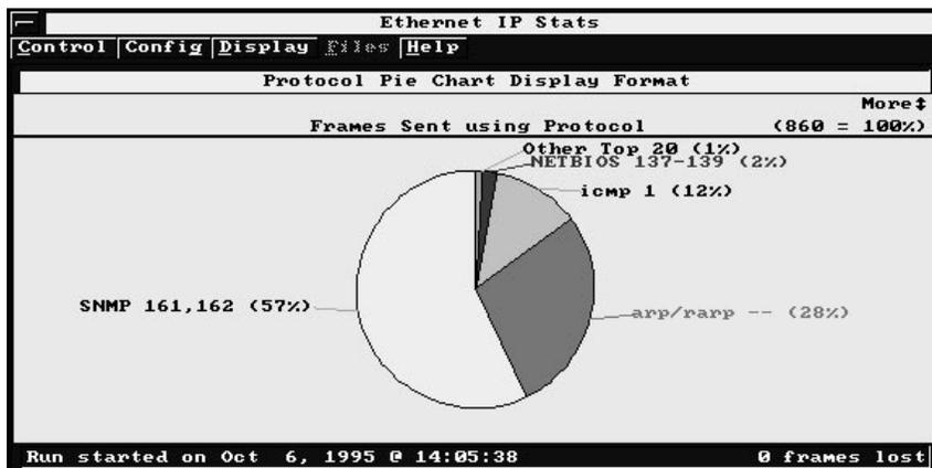
The Protocol Statistics measurement shows you how your network bandwidth is being consumed by each of the various protocol stacks (IP, Novell, DECnet, AppleTalk, Banyan Vines or OSI).
