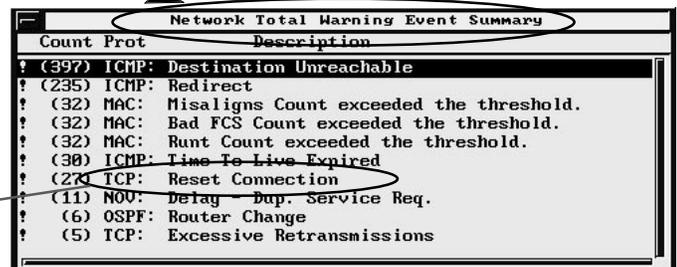
By drilling down on warning events, you can focus on inefficiencies that could be impacting network performance.
