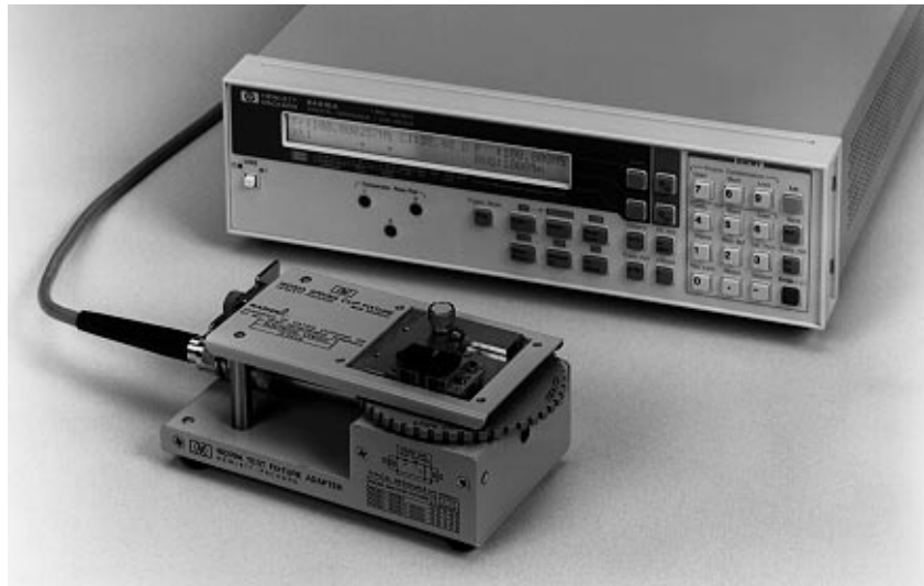
HP E4916A with opt. 001 and 010, HP 16099A and HP 16092A for LCR component measurement
