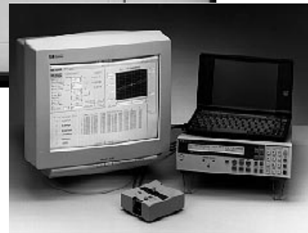
Compact crystal test system using HP E4916A, HP 41902A, and Omnibook.
