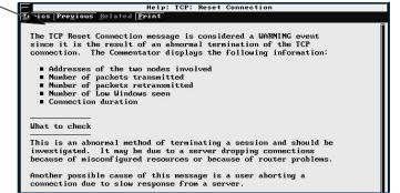
Double clicking on the event description provides an explanation of how that event was detected, its likely causes, and what to check next to resolve it quickly.
