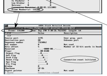
Double-clicking on the frame number(s) details the actual data frames that caused the event.
