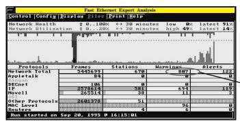
Each warning event is time-stamped and detailed, showing which stations were involved and what caused the error.
