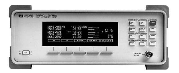
The HP 86120B Multi-Wavelength Meter is a Michelson interferometer-based instrument that measures wavelength and optical power of laser light in the 700 to 1650 nm wavelength range. Simultaneous measurements of multiple laser lines are performed allowing measurements of WDM (wavelength division multiplexed) signals and multiple lines of Fabry-Perot lasers. Each laser line is assumed to have a linewidth of less than 10 GHz.
