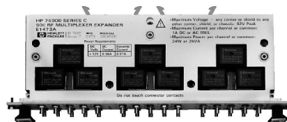
HP E1475A expander module top view
