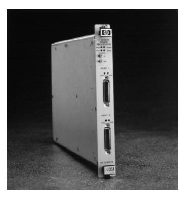
The E4207 Frame Processor is a high-performance hardware module that tests frame-based protocols at speeds up to 4 Mb/s. Two integrated V interfaces and internal RISC-based protocol test engines can each monitor, capture traffic, and generate statistics -- even with heavily loaded links and short frame lengths. The E4207 can also provide sophisticated traffic generation functionality when used with optional test software applications.
