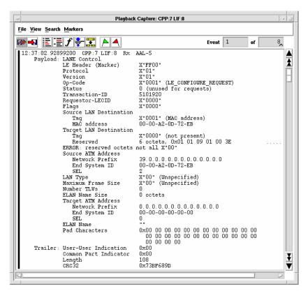
Traffic captured from local area networks emulated over ATM networks is decoded and displayed as per ATM Forum standards.
