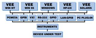
HP VEE can talk to a broad range of instruments through direct I/O, the 450 VEE drivers or any industry standard VXI plug&play driver!
