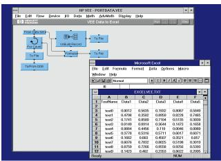
This HP VEE program uses DDE to send test data to a Microsoft Excel spreadsheet automatically.
