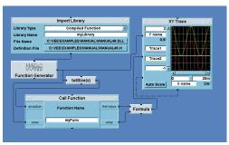
This HP VEE program is calling a C function in a DLL, which adds one to the incoming waveform and returns it to HP VEE.
