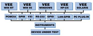
HP VEE can talk to a broad range of instruments through direct I/O, the 450 VEE drivers or any industry standard VXI plug&play driver!
