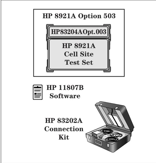
Sample order for AMPS/NAMPS cell site testing with software, training, a connection kit, a 12-month software update service contract, and a three-year return repair service contract.
