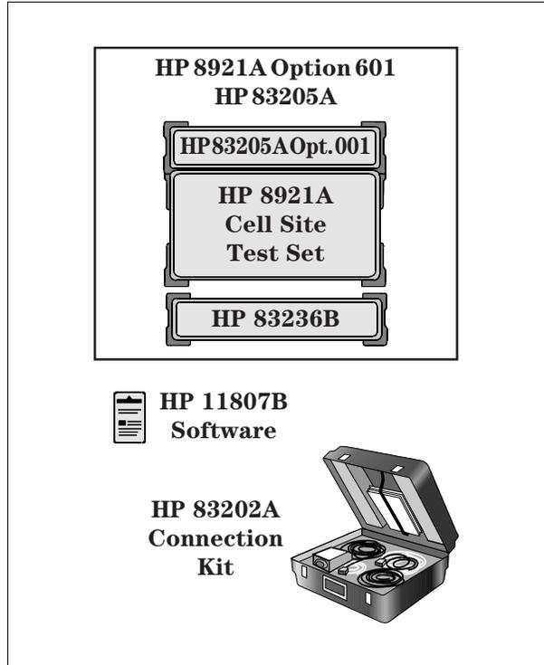
Sample order for PCS (1850 to 1990 MHz) CDMA cell site testing with a three-year return repair service contract.
