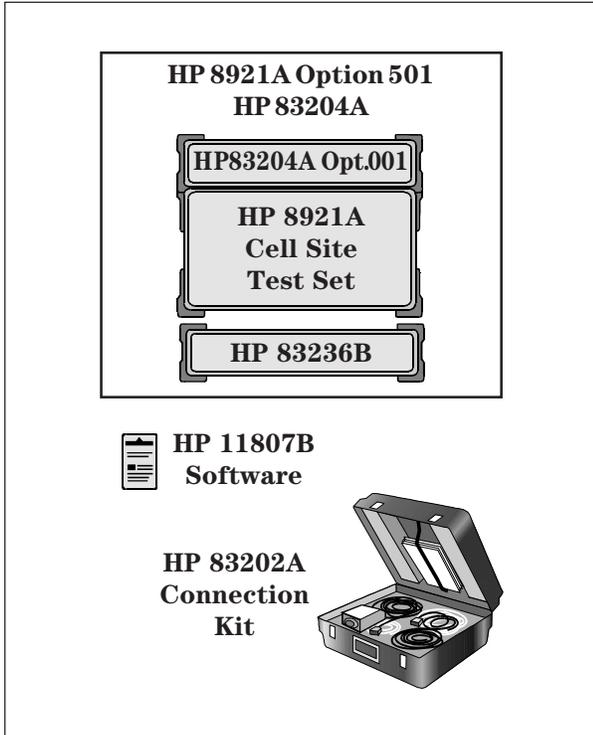
Sample order for PCS (1850 to 1990 MHz) TDMA cell site testing with a three-year return repair service contract.
