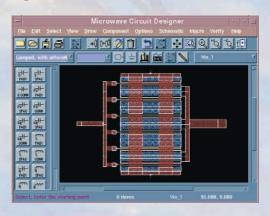
Using the Graphical Cell Compiler, static structures may be imported using the GDSII format and converted into parameterized structures such as this FET definable in terms of the number of fingers and finger width.
