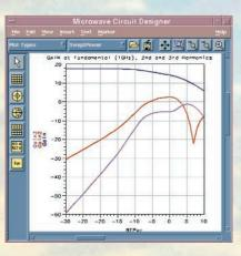
Simulate nonlinear effects such as oscillator start-up transients, amplifier compression, and multi-tone inputs. Use Microwave Circuit Designer's extensive library of microwave system, circuit, and layout elements to define the prototype from the bottom up. System-level behavioral elements include mixers, filters, amplifiers, and switches as well as models for microstrip, stripline, coplanar waveguide, and suspended substrate components.
