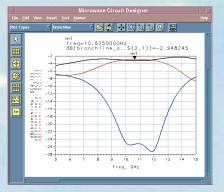
EM field simulators are traditionally used for analyzing and verifying designs, typically near the end of the design phase. Electromagnetic field optimization software from Agilent EEsof EDA offers automatic design refinement combined with EM accuracy. After the engineer specifies performance goals, the design parameters are then optimized and the final design is generated.
