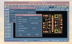
Physical design data can be easily output to a variety of convenient file formats, including Gerber, DXF, IGES, and GDSII files.
