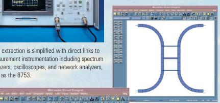
From the Microwave Circuit Designer layout window you can launch the optional Momentum EM simulator to precisely analyze complex structures.
