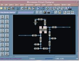
For those who require the runtime efficiency of a compiled model, the Analog Model Development Kit provides a userfriendly wizard that compiles and links model code and creates the symbols and parameter description files for use in the Microwave Circuit Designer environment.
