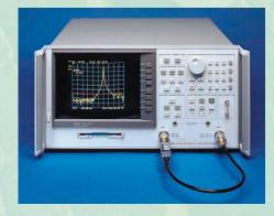
Data extraction is simplified with direct links to measurement instrumentation including spectrum analyzers, oscilloscopes, and network analyzers, such as the Agilent 8753.
