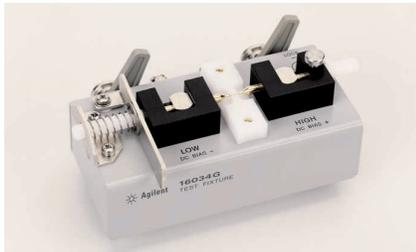
A chip component test fixture with 2-terminal configuration. The Agilent 16034G can handle small SMDs down to 0.6 mm × 0.3 mm.
