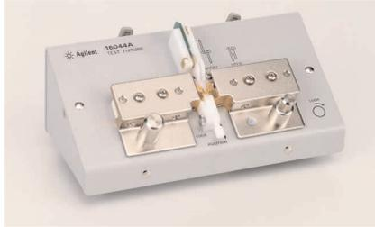
A chip component test fixture with 4-terminal configuration suited for measurement of low impedance devices such as high-value capacitors. Built-in arm-type terminators make it possible to configure appropriate terminal connections easily and quickly for Open/Short compensations by simply turning the arms.
