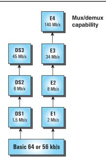
Adds T-carrier and En test capability. Testing can be performed directly at DSn/En physical interfaces or on SONET mapped payload signals.
