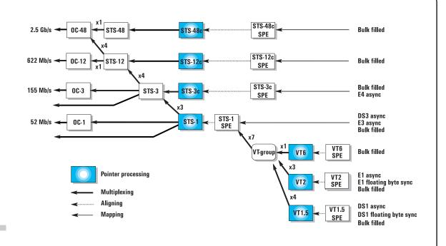
Figure 1: Bellcore GR-253 mapping structure (SONET payload mapping)
