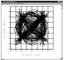
CDMA simulation results can be analyzed with a flexible set of mathematical expressions and displayed in a variety of formats including eye diagrams, constellations, spectrums, and more.
