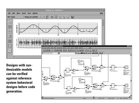
CDMA algorithms can easily be implemented with synthesizable models that allow you to automatically generate HDL code.
