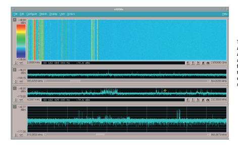
Tailor the way the Agilent E3238 presents signals. Activate up to four displays and show a spectrum trace, full-color spectrogram or two-color spectrogram in each of them, all at the same time.
