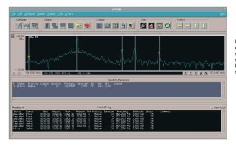
Mouse-based hand-off receiver control makes tuning to a suspect signal quick and simple. The hand-off receiver log automatically lists all the signals examined.
