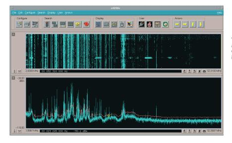
The active noise-riding auto threshold is useful when the noise floor is contoured or changing.
