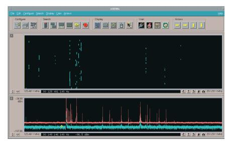
The environment threshold subtracts ambient signals and noise from the Agilent E3238 display and simplifies the task of finding new signals.
