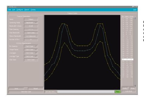
Option ASM can create limit line spectrum shapes from real signal data. C code is automatically generated to implement them.
