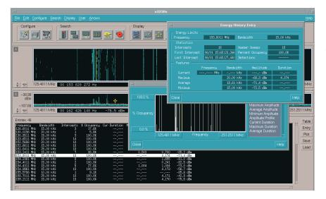
The energy history database automatically stores the parameters of all energy above the threshold.
