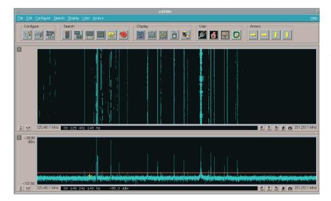
The level threshold is simple and effective with a flat noise floor.
