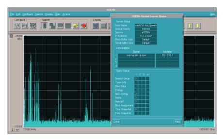
The Agilent E3238 uses UNIX sockets for powerful connectivity.
