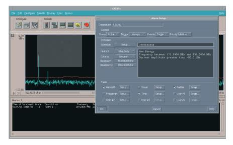
Automatically classify the energy in the energy history database with the alarm function.
