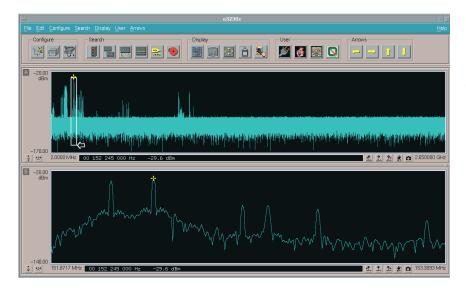
Zooming the display on a signal is simple with the Agilent E3238. It keeps sweeping while the selected area is zoomed. The lower trace shows the zoomed display, the upper is the full measured spectrum.
