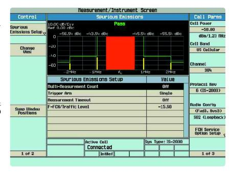
The test application performs extremely fast cdma2000, IS-95, and AMPS transmitter and receiver tests using call processing to establish a traffic or fundamental channel via standard test service options or in test modes for mobile phone calibration.
