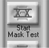
13. The mask will automatically align to the waveform and the measurement results will appear in the measurement tab window. Waveforms which were taken prior to the start of the mask test are included in the results. To clear all waveforms and start a mask test with entirely new data press the Clear Display hardkey (near the floppy disk drive). If you would like to scale or position the mask manually, push the Mask Test Scaling soft key in the scroll window on the left.
