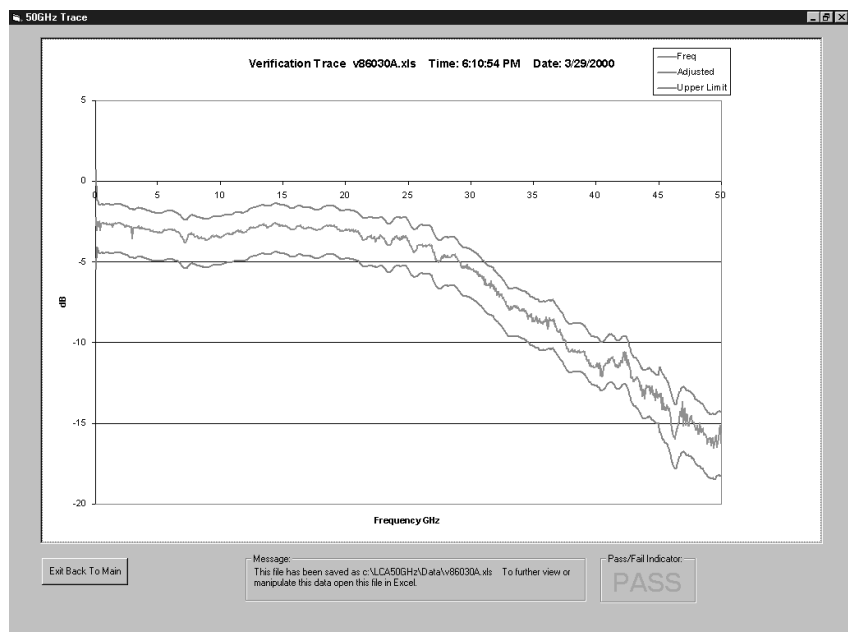
Figure 1. Typical verification device measured data, with tolerance limit lines.
