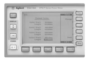
Versatile user interface displays up to four time gates and lengths in a single measurement setup. This menu is accessed using the CHANNEL hardkey.
