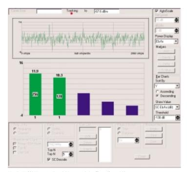
Use the W-CDMA receiver-based drive test solution (E7476A) to quickly troubleshoot base station timing and drift errors by measuring the chip offsets of each sector of a base station.
