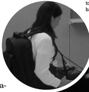
A pouch on the side of the backpack allows two phones to be carried with the system. Alternatively, for phone based measurements only, the pen-tablet computer and phones can be used without the backpack and receiver configuration.
