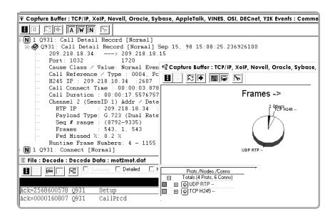
A distinct advantage of the Advisor with Voice is its ability to analyze in realtime as well as in Post-Analysis Mode. The Post-Analysis method involves attaching the analyzer to the network, capturing data for a period of time, and then stopping the analyzer. The analysis is then performed OFF LINE, while no more data is taken from the line. This is a time consuming process, especially when the problem packet is not found in the capture buffer.
