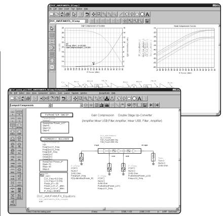
The RF System DesignGuide from Agilent EEsof EDA works with Advanced Design System to configure transmitter and receiver chains using behavioral system models.
