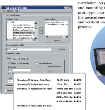
PA Design Director dialogs guide you through test set-up. Batching up sequences of tests frees your time for other tasks. Results output is ready for your electronic lab notebook.
