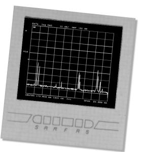
The total return loss of this photodiode assembly is due to several different interfaces. The 8504B precision reflectometer shows the return loss of each of the photodiode's elements. Designers no longer need to guess where to concentrate their efforts in improving the product.
