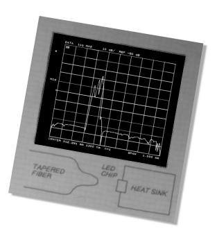
Return loss is also an important parameter for lightwave sources. Light reflected from components beyond the laser or LED source can be re-reflected off of the source leading to distorion in analog communications systems and bit errors in digital systems.
